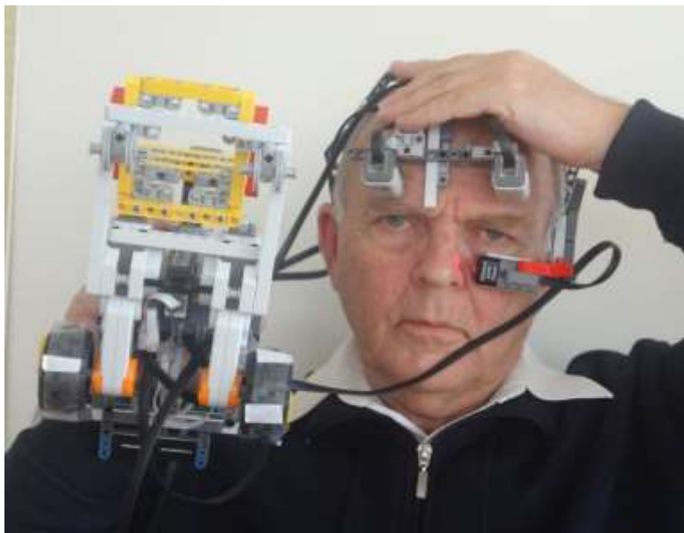
Fig. 2: Prototype wheelchair control with head movements.
