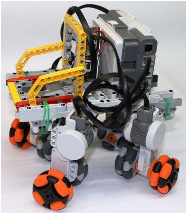
Fig. 5: A holonomic wheelchair prototype.
